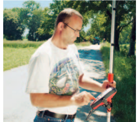
The SR20 being used to collect centimeter accurate topographic data using kinematic techniques.
